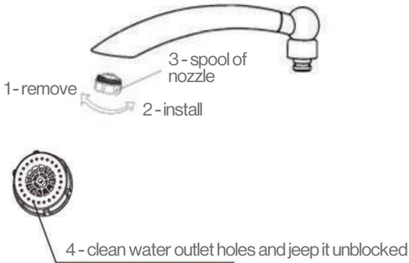
Cleaning of water filter: If the water flow becomes small after being used for period of time, remove and clean filter as indicated in the picture below, and assemble back in turn.
